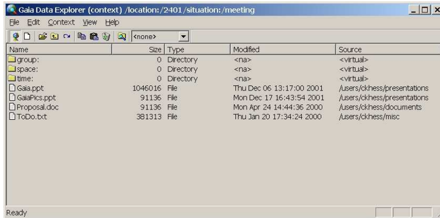
Fig. 3. Screenshot of the context file system browser. The virtual hierarchy is used to attach context to files and directories
